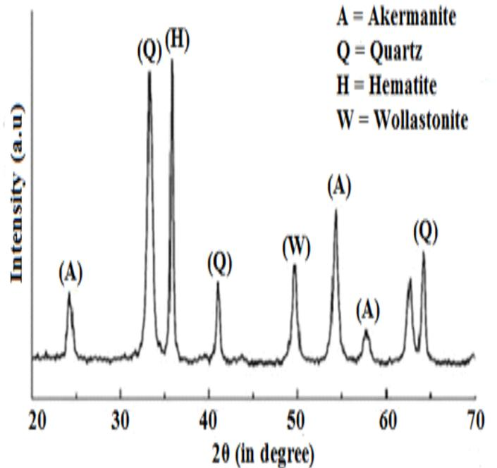
Fig. 4. XRD of air cooled slag
