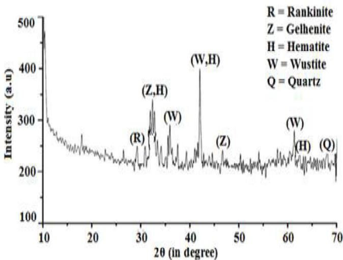
Fig. 3. XRD of granulated slag
