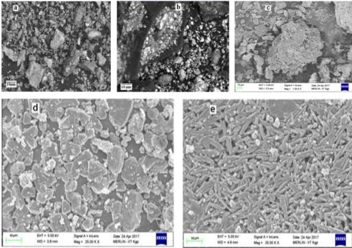
Fig.2.SEM of granulated slag (a), air cooled slag (b), SMS slag (c), SMS sludge (d) and fly ash (e)
